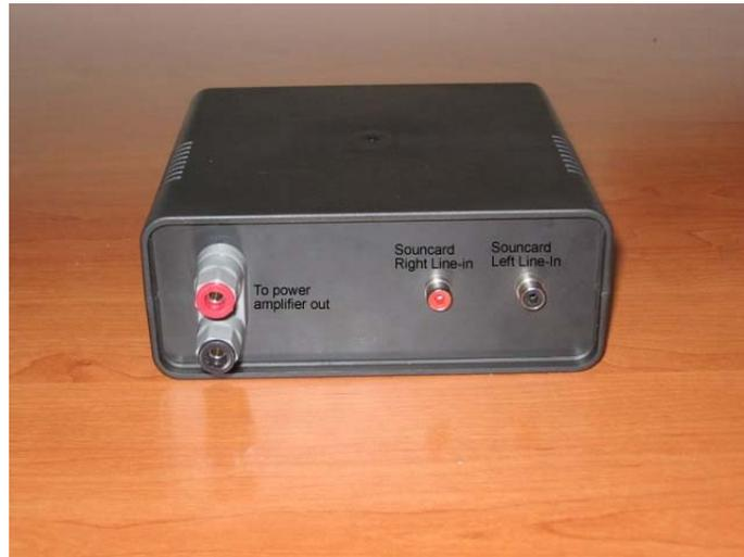
Figure 2. Back view of the MeasuringBox.
